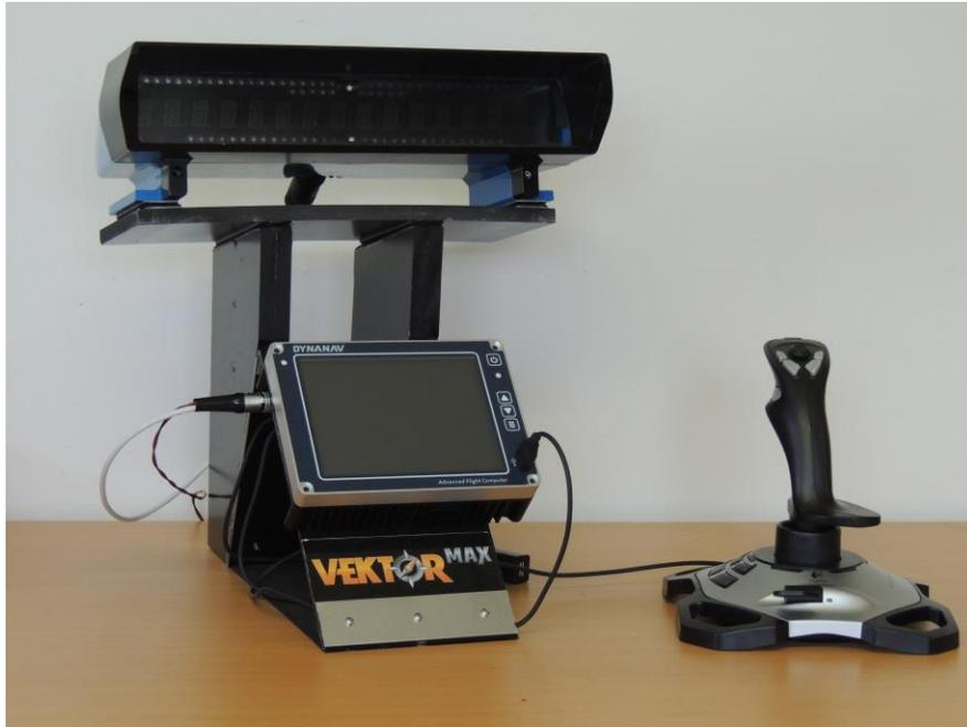
Start by connecting the Joystick into the frontal USB port of the Vektor MAX system.
